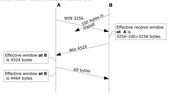
The window size is a *flow control mechanism* by the *receiver*. It makes the sender send only as many bytes as the receiver is prepared to accept, thereby not overwhelming the receiver.
