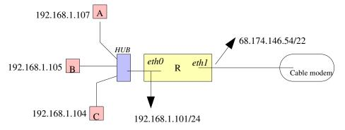
This is a set up you can use if you do not have a commercial Cable/DSL router. In fact, home routers are simple machines like R in the figure above, running linux and a web server for system administration.
