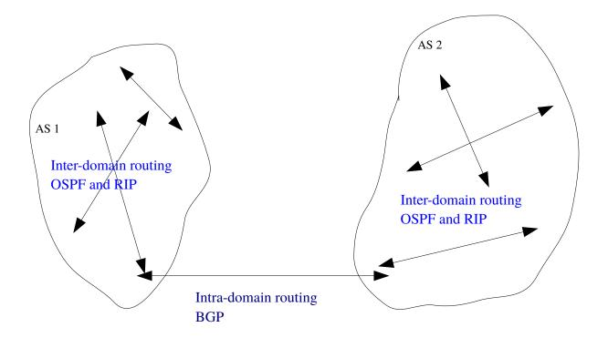
In general, most routing within Autonomous Systems use Routing Information Protocol (RIP), or its enhanced version Open Shortest Path First (OSPF). The current de facto Intra-domain routing standard is Border Gateway Protocol(BGP), Version 4 (<u>RFC 4271</u>). You need to concern yourself with these protocols if you are dealing with routers inside or between Autonomous Systems.
