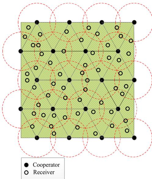
Fig. 2 The network model of EHC-WSN
