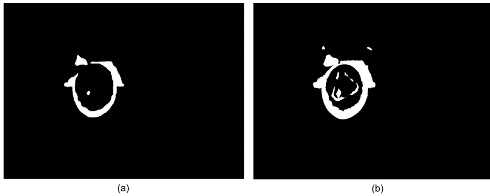
Fig. 7. Binary masks, where white pixels represent areas of oil stains and black pixels represent background. Image (a) shows the segmentation results of the original image in Fig. 8 predicted by the one-stage model, and (b) shows a ground-truth mask.
