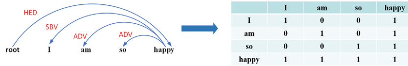
Fig. 3. Dependent syntactic structure analysis and its corresponding adjacency matrix. HED stands for a core relationship, SBV stands for a subject-predicate relationship, and ADV stands for an adverbial relationship.
