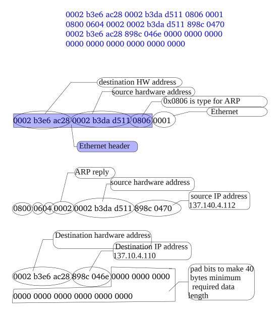
This is a reply from 137.140.4.112 to 137.140.4.110 saying that "137.140.4.112 is at 00:02:b3:da:d5:11". This must be in reply to an ARP request broadcast from 137.140.4.110 asking "who has 137.140.4.112, tell 137.140.4.110".
