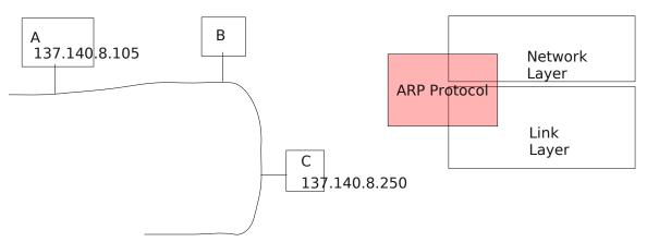
In order to find the MAC address of C, A's ARP broadcasts an ARP request, basically asking "who has the IP 137.140.8.250? Tell 137.140.8.105". All hosts on the network will receive this ARP request broadcast.
