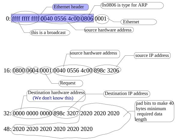
This is an ARP request from interface with IP address 137.140.50.6 to
